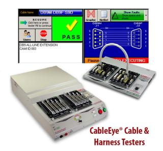
CAMI Research produces expandable and upgradable diagnostic Cable & Harness Test Systems for assembly, prototyping, production, and QC of standard or custom cables. CableEye® Testers display, and document basic electrical properties such as continuity, resistance, dielectric breakdown, insulation resistance, miswires, and intermittent defects. camiresearch.com
