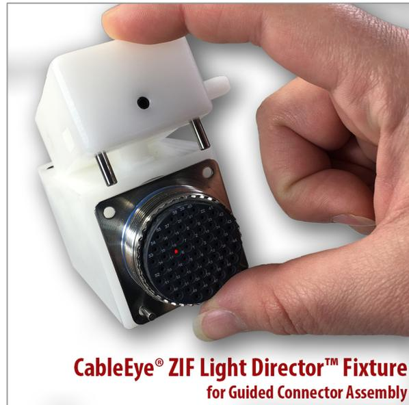
**Fixture shown with connector to be assembled being locked in place, and a pin location illuminated.**
